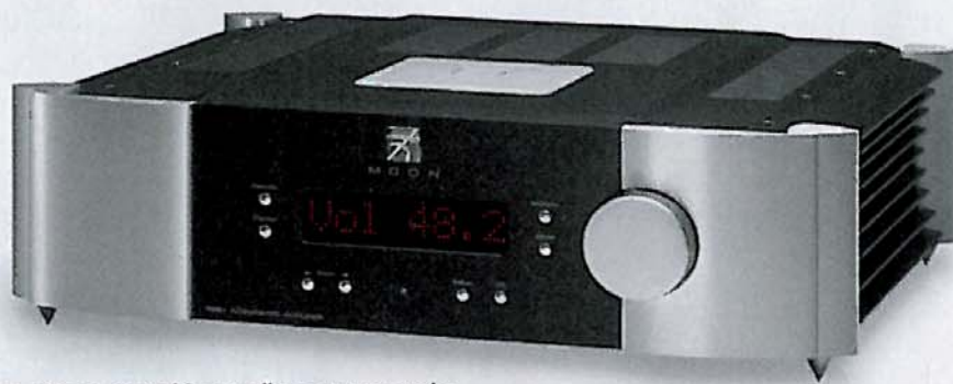
The volume control is actually a rotary encoder controlling Simaudio's proprietary M-eVOL2 circuit.
