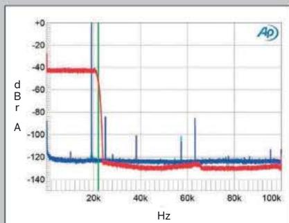
**Fig.1** Simaudio Moon Neo 340i, S/PDIF input, wideband spectrum of white noise at -4dBFS (left channel red, right magenta) and 19.1kHz tone at 0dBFS (left blue, right cyan), with data sampled at 44.1kHz (20dB/vertical div.).
