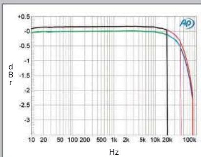
**Fig.2** Simaudio Moon Neo 340i, S/PDIF input, frequency response at -12dBFS into 100k ohms with data sampled at: 44.1kHz (left channel gray, right green), 96kHz (left cyan, right magenta), 192kHz (left blue, right red) (0.5dB/vertical div.).
