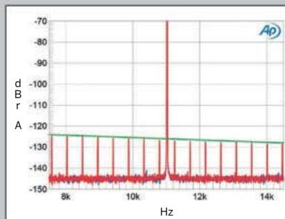
**Fig.5** Simaudio Moon Neo 340i, S/PDIF input, high-resolution jitter spectrum of analog output signal, 11.025kHz at -6dBFS, sampled at 44.1kHz with LSB toggled at 229Hz: 16-bit data (left channel blue, right red). Center frequency of trace, 11.025kHz; frequency range,  $\pm 3.5$ kHz.
