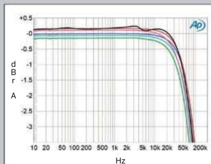
**Fig.8** Simaudio Moon Neo 340i, unbalanced frequency response at 2.83V into: simulated loudspeaker load (gray), 8 ohms (left channel blue, right red), 4 ohms (left cyan, right magenta), 2 ohms (red) (0.5dB/vertical div.).
