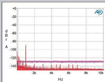
**Fig.3** Simaudio Moon Neo 340i, S/PDIF input, 44.1kHz data, spectrum with noise and spuriae of dithered 1kHz tone at -90dBFS with 16-bit data (left channel cyan, right magenta), 24-bit data (left blue, right red) (20dB/vertical div.).
